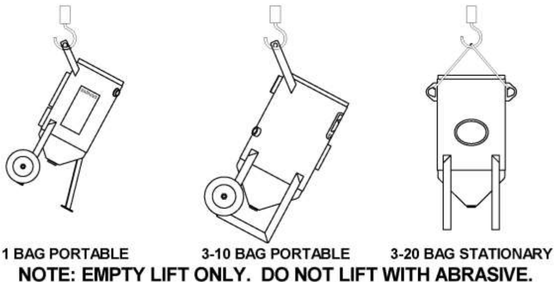
Figure 2.6(a) – Abrasive Blaster Lifting Diagram
