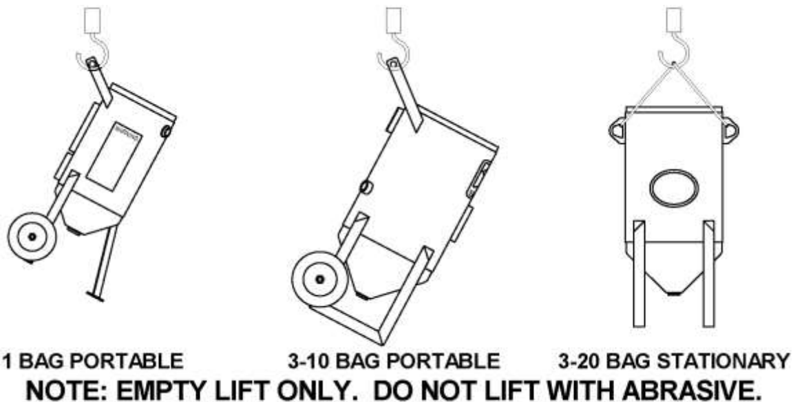
Figure 2.6(a) – Abrasive Blaster Lifting Diagram
