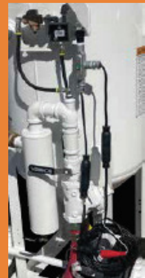
Blast Pot before conversion
